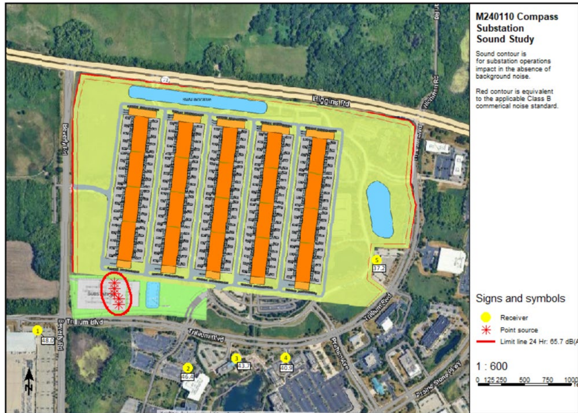
Figure 5. A Weighted Sound Pressure Level Impacts for COMPASS Hoffman Estates. Red Contour is Extent of 65.7 dB(A) Equivalent Impact for Comparison to Standard.
